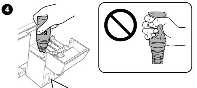
Ink flow stops automatically when the ink level reaches the upper line.
